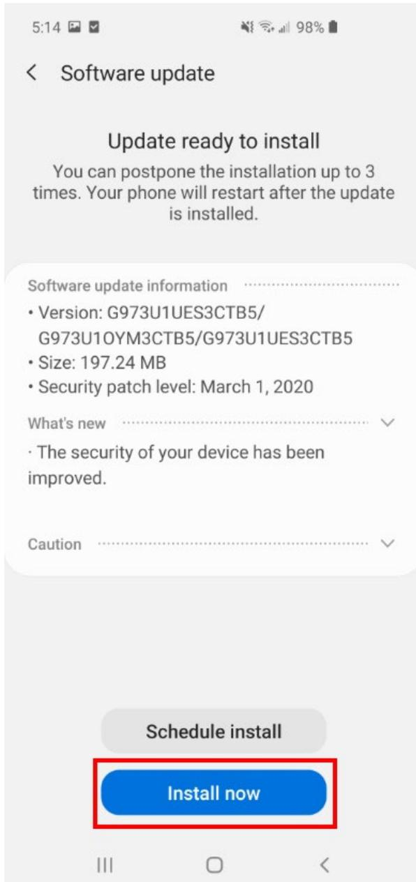
7. The device may reboot during the update process. Once the update is complete, the device will return to the lock screen.
